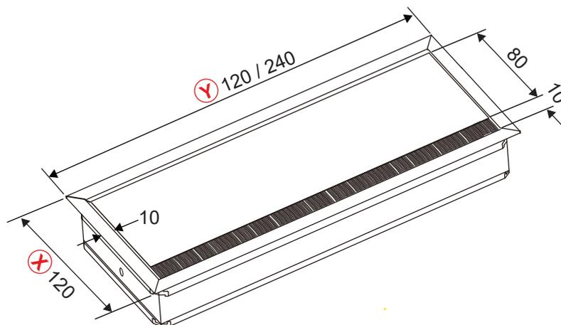
Cable passage dimension (underside)  $A = X - 36$
