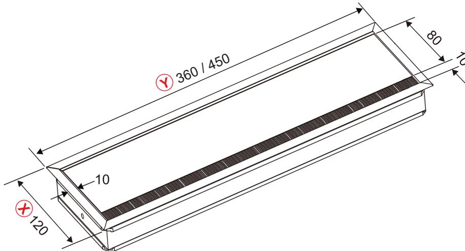
Cable passage dimension (underside)
