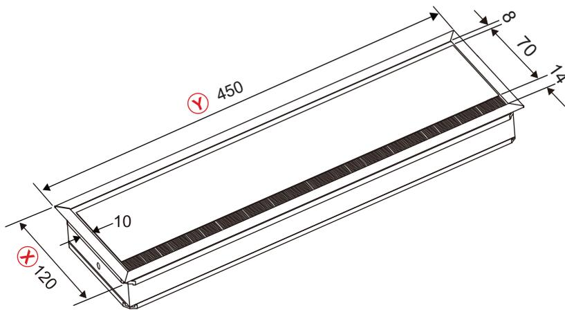
Cable passage dimension (underside)  $A = X - 36$
