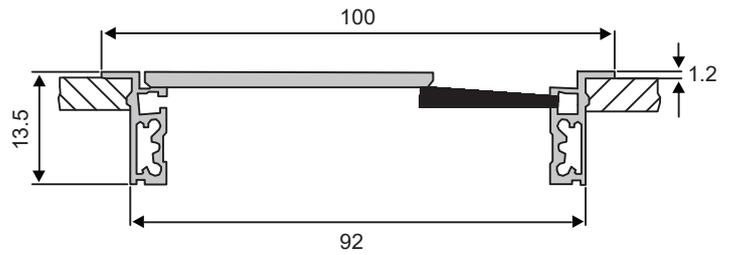
Cable passage dimension (underside)  $\textcircled{A} = \textcircled{X} - 32$
